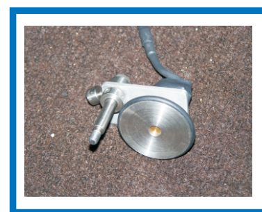
PRO-MIC Encoder Assembly for Distance Measurement
